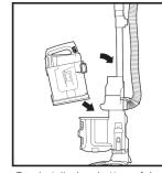
To reinstall, place bottom of dust cup into pod and then tilt back until it clicks into place.
