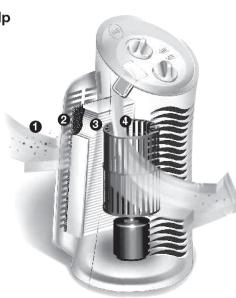
1 From the air that passes through the filter, 2 microns and larger. Overall particle reduction depends on many factors including the amount of air processed, the pollutant type, and the pollutant's introduction rate into the environment.
