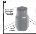
4 Set up the air purifier on a flat. level. floor surface, at least 3 inches (8 cm) away from walls and objects. If included with your HP300 series air purifier, locate the odor neutralizer technology cartridge and follow the instructions for how to insert into the product.
