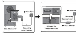
Make sure to rest the AC/DC Adapter flat on a table or the floor. If you place the AC/DC Adapter so that it is hanging with the AC cord input facing upwards, water or other foreign substances could the Adapter and cause the Adapter to malfunctior
