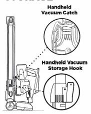
Press the Wand Release button on the top of the wand to release the handheld vacuum. There is a catch on the bottom of the handheld vacuum. Hang it from the hook located on the bottom portion of the wand. Wrap the cord around the two cord hooks.
