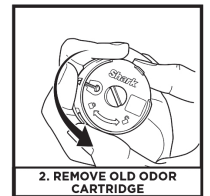
2. REMOVE OLD ODOR CARTRIDGE
