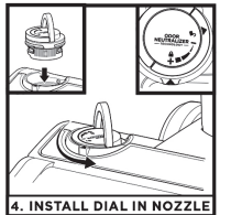
4. INSTALL DIAL IN NOZZLE
