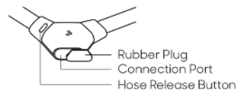
Air Hose Extension (Top View)
