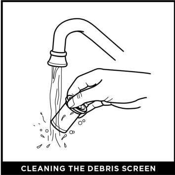
CLEANING THE DEBRIS SCREEN
